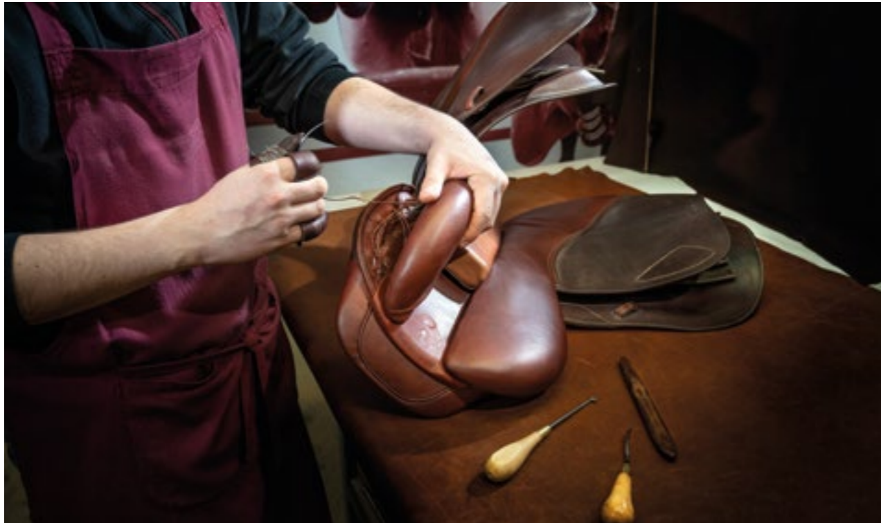
To avoid using chrome, LIM has revived an age-old, 100% veg-tanning process in which the hides are rotated in large tanning drums containing three different types of bark (see above). Once prepared, the leather is transported to CWD's site in Nontron to make saddles. Here, a stitching awl and heavy, waxy thread (known as "poissé" in French) are used to lace the leather (below). The artisan protects their hands with leather finger protectors on the index and little fingers.
