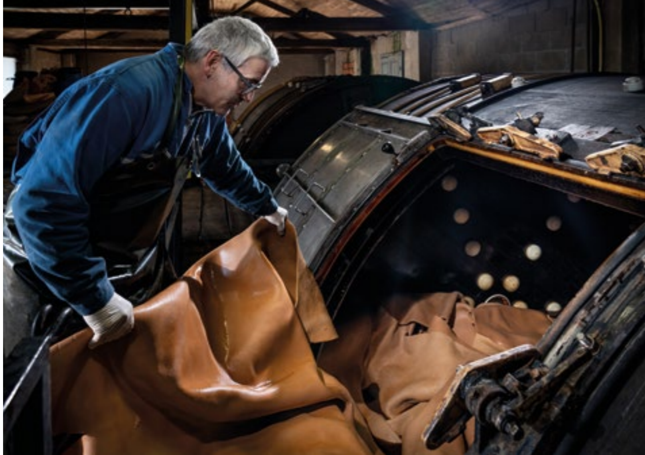
To avoid using chrome, LIM has revived an age-old, 100% veg-tanning process in which the hides are rotated in large tanning drums containing three different types of bark (see above). Once prepared, the leather is transported to CWD's site in Nontron to make saddles. Here, a stitching awl and heavy, waxy thread (known as "poissé" in French) are used to lace the leather (below). The artisan protects their hands with leather finger protectors on the index and little fingers.
